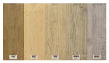
Brushed spruce matchboards. The final colour is given by the overlap of two different colours of the Lignum Terradilegno colour range (from left to right: Sand + Mud, Clay + Sand, Mud + Sand, Anthracite + Sand, Anthracite + Dolomite).
